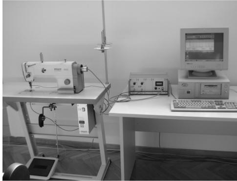
Figure 1 - Instrument for needle stitch force measurement
